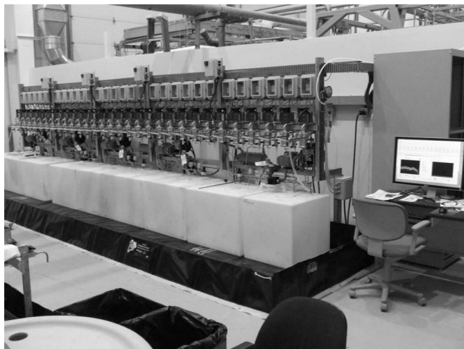
FIG. 1. Thirty Stage centrifugal contactor pilot plant.
